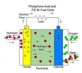
Figure 5.10. The working principle of PAFC and PEM fuel cells (Smithsonian 2001).
