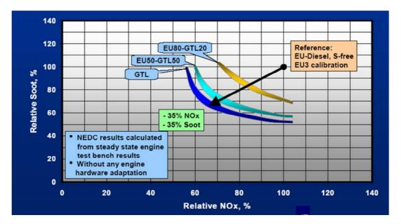
Figure 6.11. The effect of GTL diesel on passenger car  $NO_x$  and PM emissions (Maly 2004).
