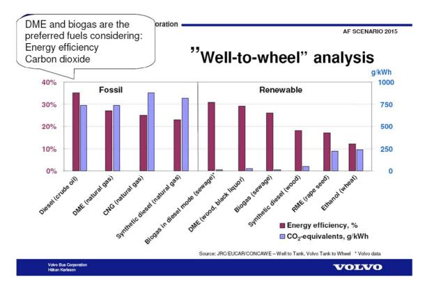
Figure 7.6. Well-to-wheel energy efficiency and  $CO_2$  emissions of various fuels (Jobson 2007).
