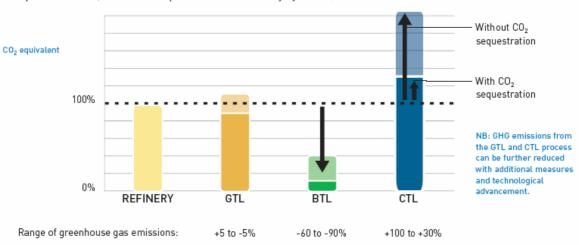
Comparison of GTL, BTL and CTL processes with refinery systems (on a well-to-wheel basis)
