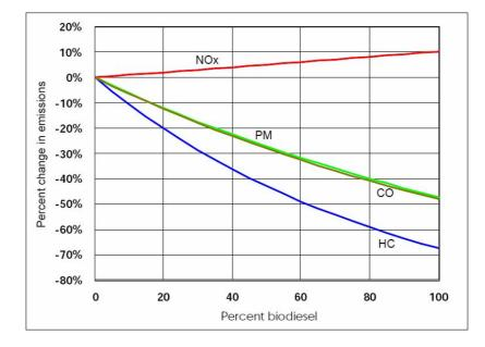
Figure 6.8. The effect of fatty acid methyl ester (biodiesel) concentration on regulated exhaust emissions (EPA 2002).
