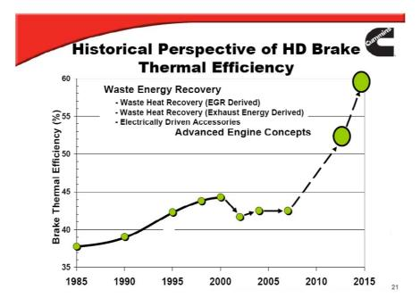
Figure 5.7. Projected increase in engine thermal efficiency (Eckerle 2007).
