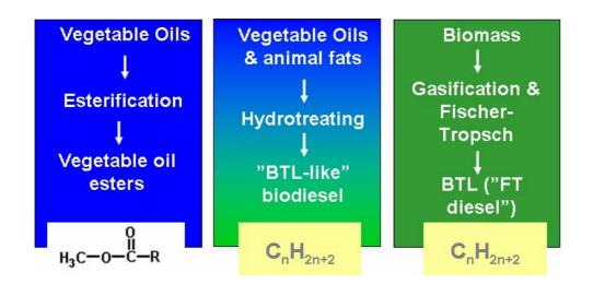
Figure 4.6. A schematic figure of the main biodiesel processes and end products.
