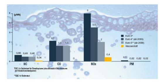
Figure 6.17. Emissions values for MAN's hydrogen ICE. Wasserstoff = hydrogen. (MAN)
