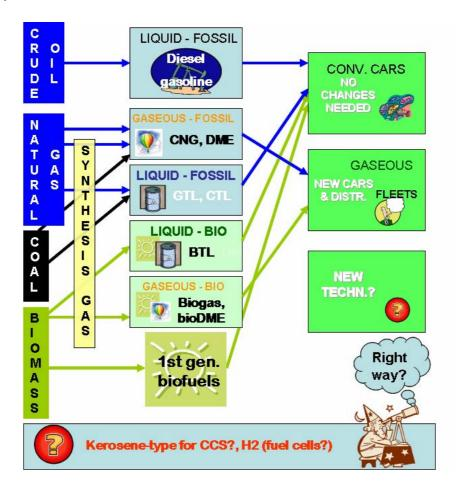
Figure 4.3. Links between feedstocks, fuels, and end-use in transportation.
