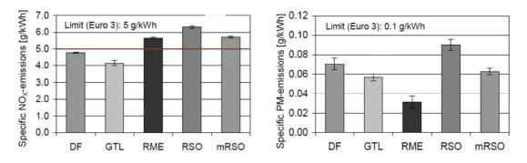
Figure 6.9.  $NO_x$  and PM emissions with diesel fuel, GTL, RME and unmodified (RSO) and modified (mRSO) straight vegetable oil (Krahl et al. 2007).
