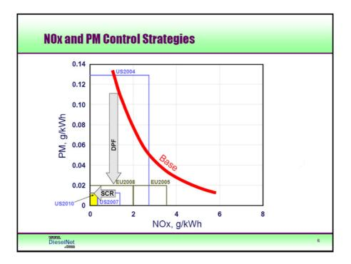
Figure 5.5. Emission reduction strategies for HD on-road vehicles. Base shows the trade-off between  $NO_x$  and PM for conventional diesel engines. (Majewski 2006)
