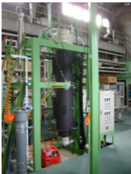
Fig.1: Lab-scale entrained biomass gasifier.
