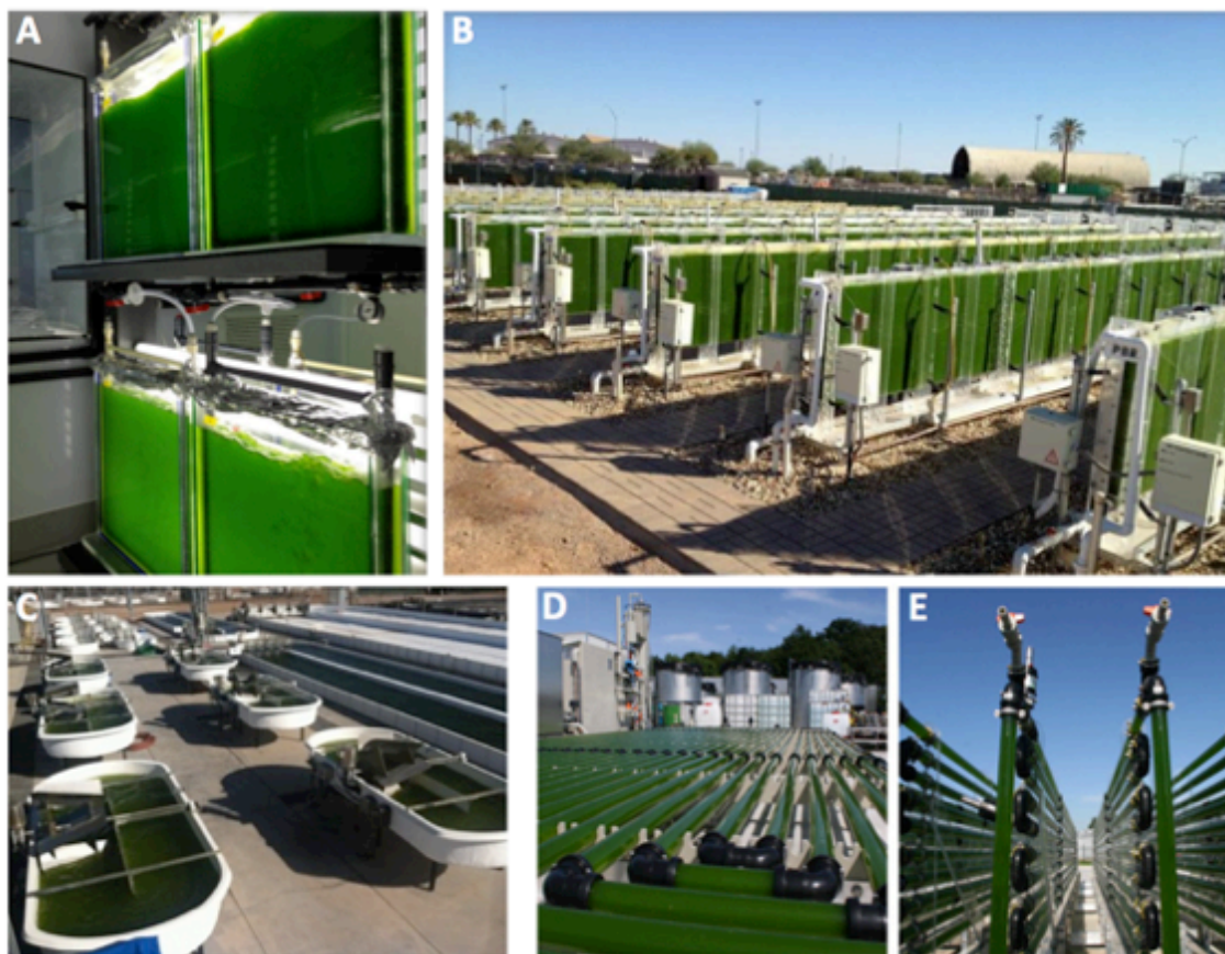
Figure 3-6: Cultivation systems for algae growth. (A-B) flat panel photobioreactors at AzCATI), 39 (C) Small, 1000 L research open ponds at AzCATI, and (D-E) horizontal and vertical tubular photobioreactors at Algae PARC (between 12m 2 and 24 m 2 each) 119
