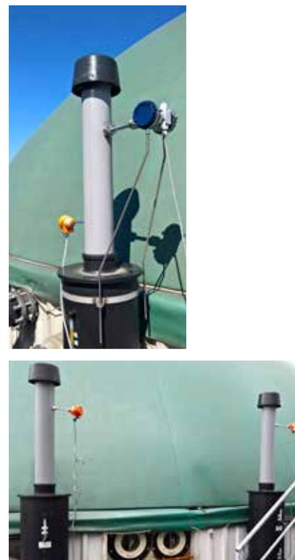
Figure 16: Measurement setup for PRV monitoring (DBFZ)
