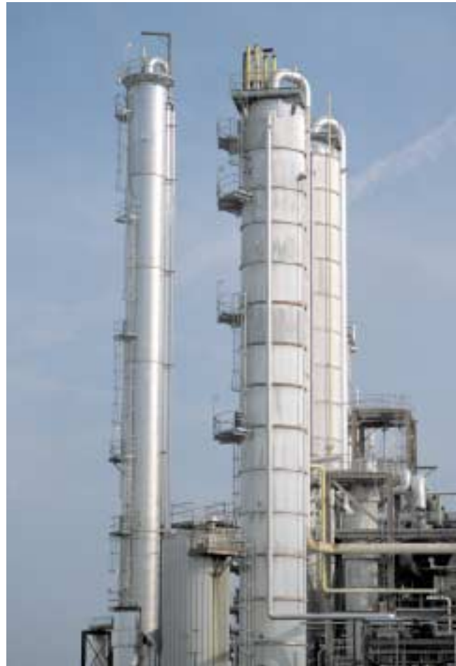
Ethanol distillation towers at the Pekin Energy Company, Illinois, USA. (Courtesy DOE/NREL and W. Gretz)
