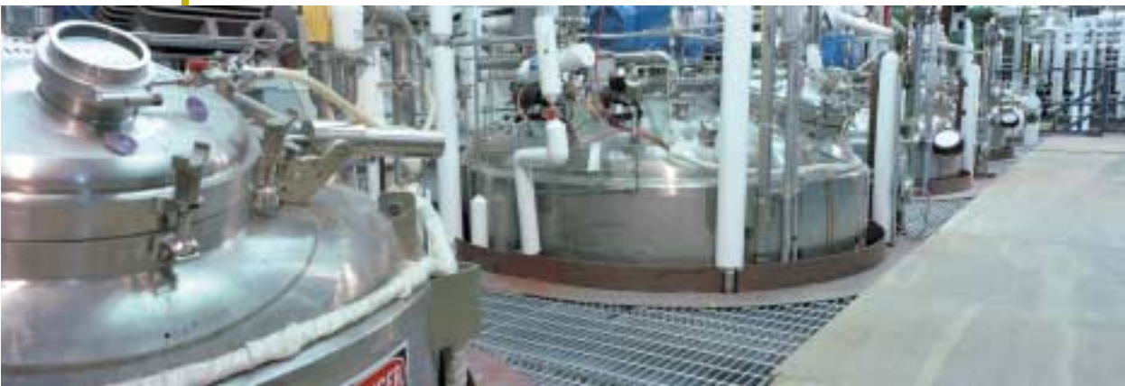
Process Development Unit for biomass to ethanol, 9000 litre fermenters, Golden, Colorado, USA. (Courtesy DOE/NREL and W. Gretz)
