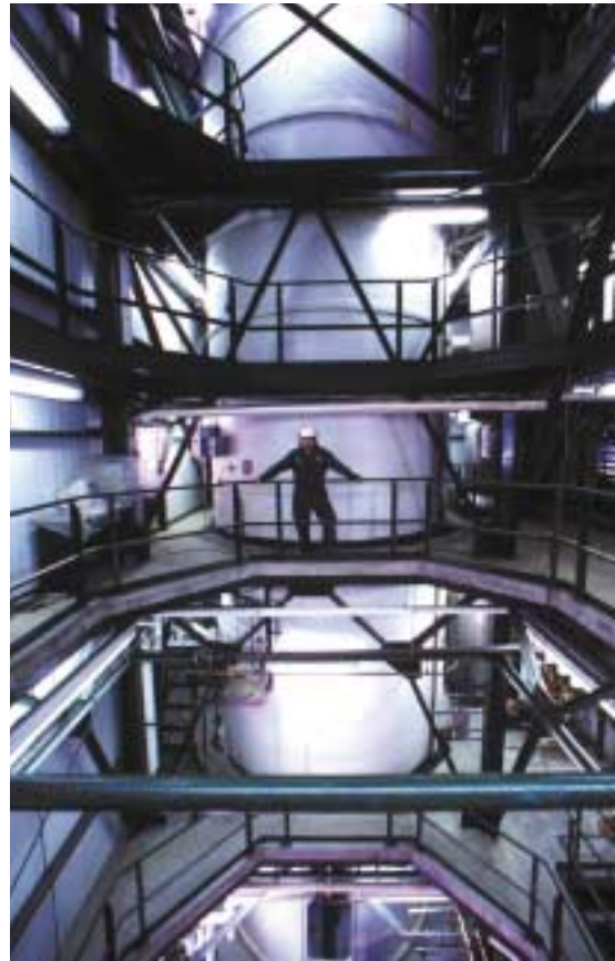
Fermentor in Iogen agricultural biomass-to-ethanol demonstration facility. (Courtesy Iogen, Canada)
