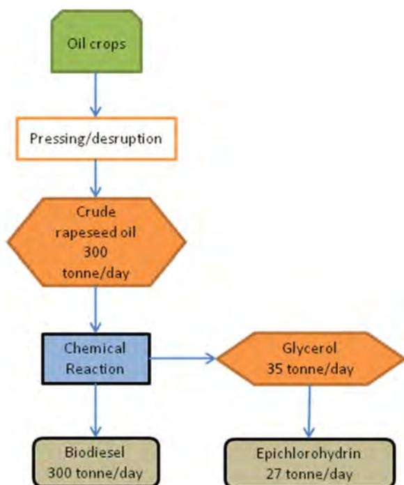
Figure 6. Integrated biodiesel and epichlorohydrin production.
