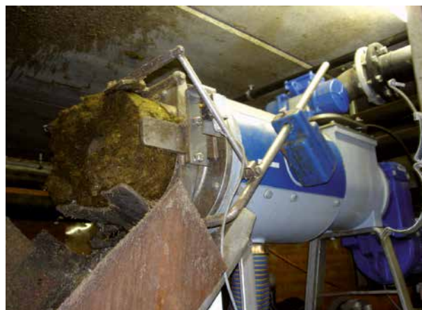
Figure 7: Screw press separator (Source: Fuchs and Drosig, 2010)
