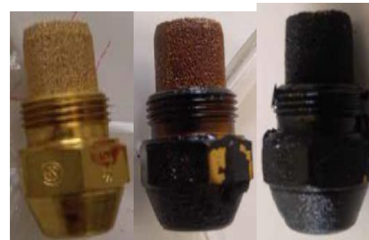
Exposure of brass nozzles to blends of upgraded bio-oil and heating oils. “Pyrolysis and Upgrading of Bio-oils Derived from US Northeast Hardwood for Application in Home Heating Oils”, TCBIomass 2015.
