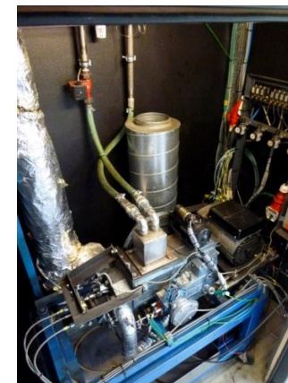
BTG has tested a 1-cylinder CI-engine, adapted to run bio-liquids including pyrolysis oil
