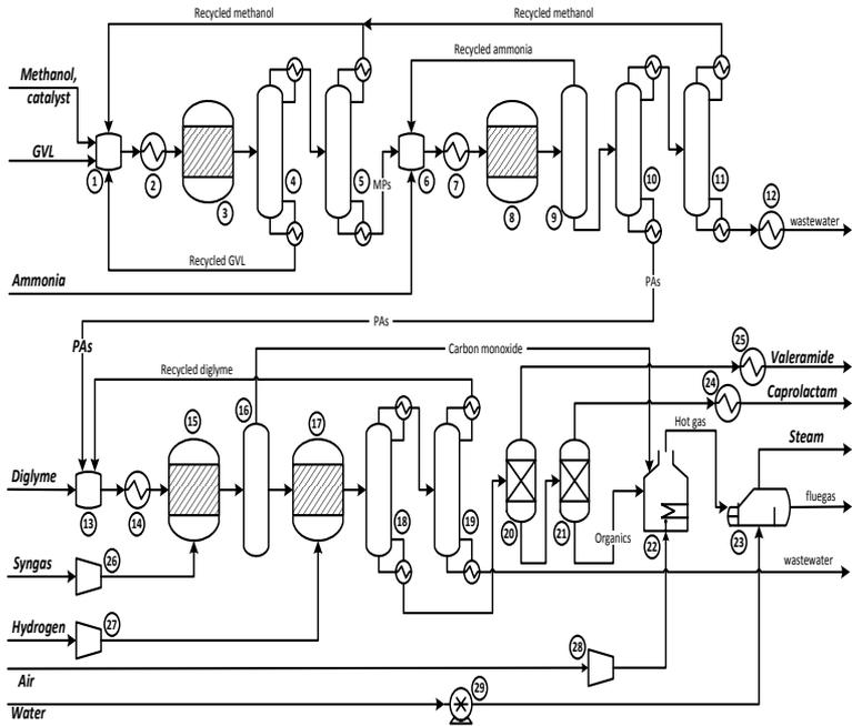
Simplified flow diagram of the production of caprolactam from  $\gamma$ -valerolactone (one out three process sections in a briorefinery concept from c6 sugars to caprolactam)
