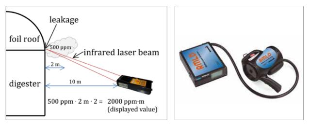
Figure 5: Use of a portable methane laser to detect leakages (left: Holmgren et al., 2015; right: Hermann Sewerin GmbH, Gütersloh)
