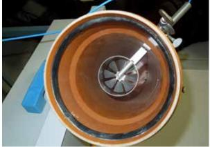
b) vane anemometer for flow measurement in point sources (DBFZ)
