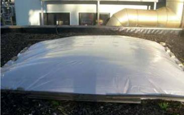
b) Measurement setup at an open biofilter [DBFZ]
