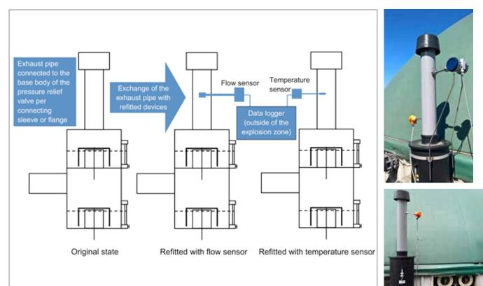
Figure 15: Schematic representation of the measurement setup for PRV monitoring (adopted from Heeren Hepolan GmbH, Schorba)
