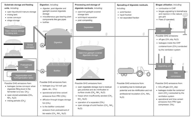
Figure 25: Overview about GHG emission sources from components and processes applied within biogas production and utilisation
