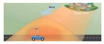
Figure 24: Schematic overview of the dynamic plume tracer dispersion method (Holmgren et al., 2015)
