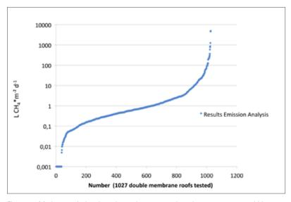
Figure 27: Methane emission through membrane covers based on measurement within air of air inflated double membrane roofs (1027 roofs measured, Clemens (2014))
