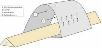
Figure 12: a) Wind tunnel for the evaluation of emissions from composting heaps treating digestate b) Wind tunnel (Phong, Nguyen, 2012)
