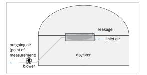
Figure 8: Methane emissions from leakage a) graphic account (DBFZ)
