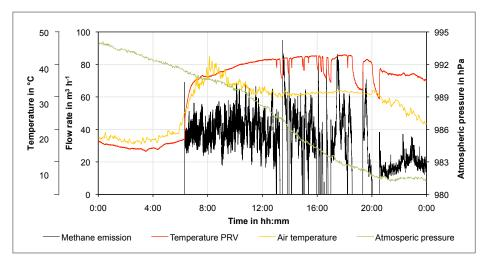
Figure 29: Influence of atmospheric conditions on the methane emissions from a PRV of a biogas plant, adopted from (Reinelt et al., 2016)
