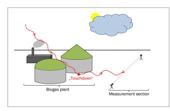
Figure 21: Schematic of the concept of WindTrax based simulation (DBFZ)
