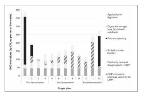
Figure 18: GHG emissions of biogas plants treating separately collected biowaste (Daniel-Gromke et al., 2015)
