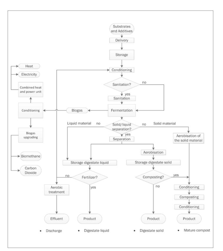
Figure 1: Possible process components and processing pathways for anaerobic digestion
