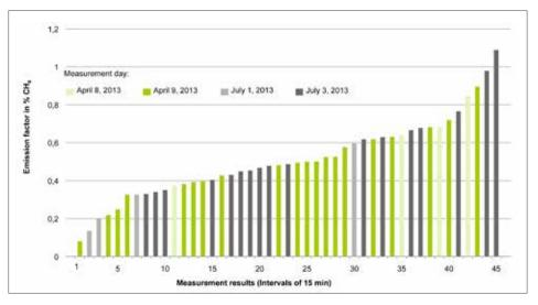
Figure 23: Emissions from a biogas plant based on open path readings (15 min average, sorted by size) and WindTrax based calculations, adopted from Westerkamp et al. (2014a).
