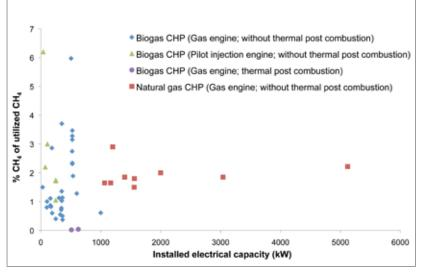
Figure 34: Methane emissions from CHP units operated with biogas and natural gas (Liebetrau et al., 2013a; Aschmann, 2014, Kretschmann et al., 2012; van Dijk, 2012)
