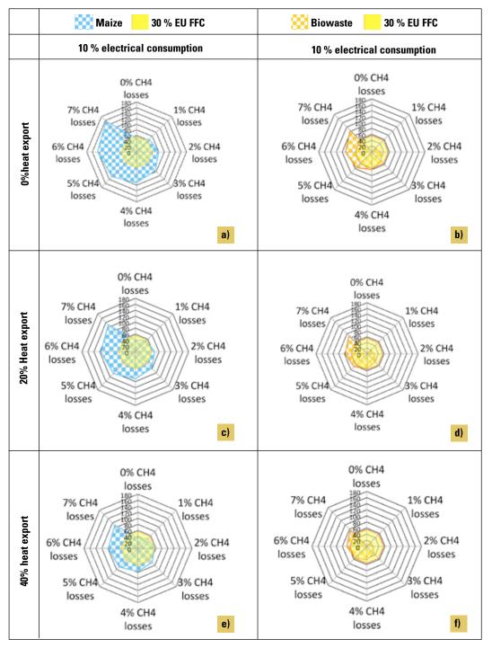
Figure 37: Impact of heat utilization and substrate on GHG emissions; plants based on maize and biowaste
