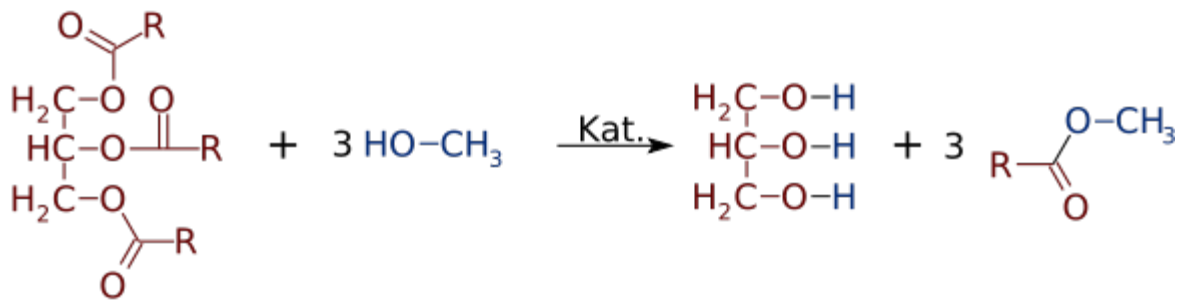
Figure 9 Transesterification of triglycerides with methanol to glycerol and methyl esters for the production of fatty acid methyl esters (FAME)
