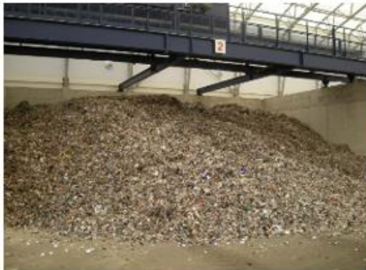
Certificated Solid Recovered Fuel (SRF) produced from biomass and household waste in the frame of the EU funded RECOMBIO project [1]
