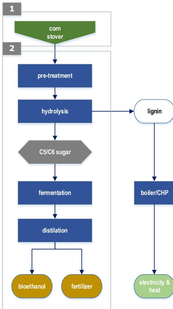
Figure 8 Case study #1: Lignocellulosic ethanol biorefinery pathway.
