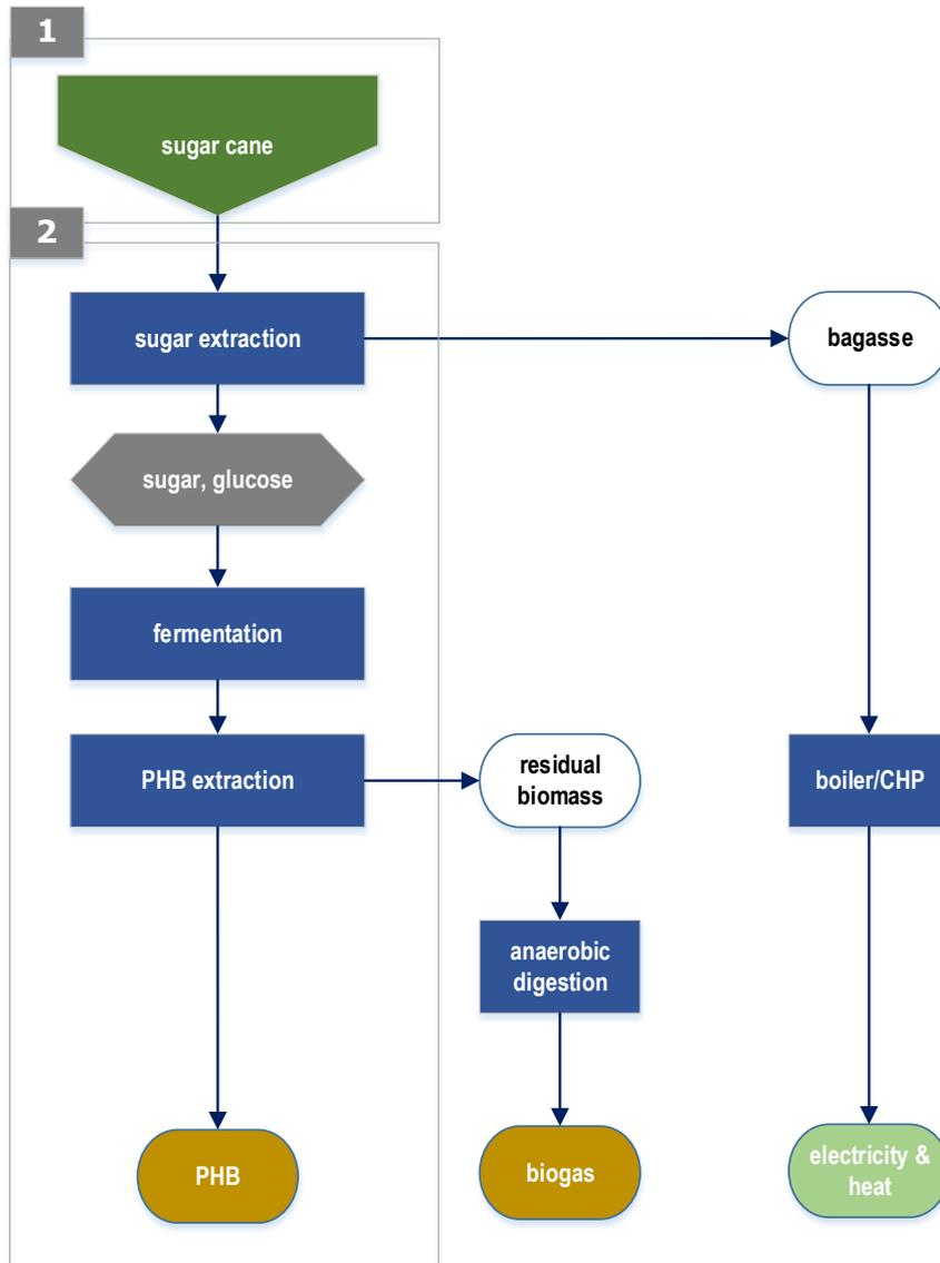
Figure 17 Poly-hydroxybutyrate (PHB) biorefinery pathway.
