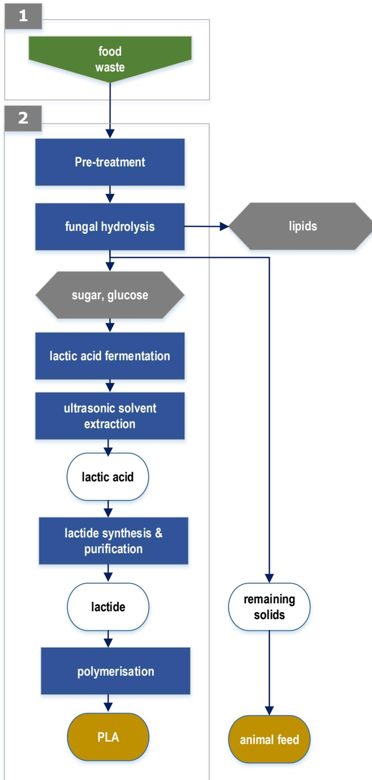
Figure 24 Process pathway PLA from waste.
