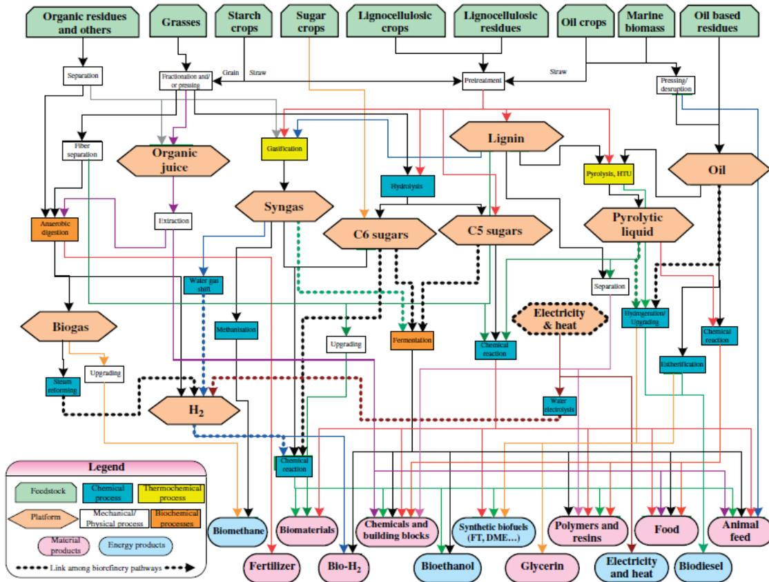
Figure 4 Network where the individual biorefinery systems are combined (Cherubini et al., 2009).
