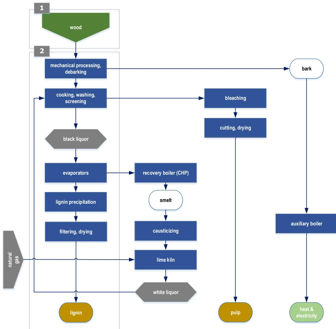
Figure 32 Lignocellulosic biorefinery pathway.
