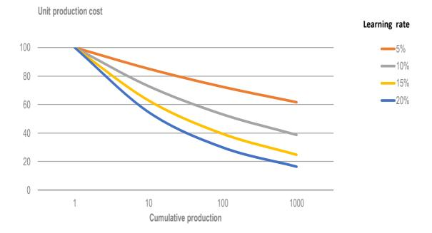
Figure 11. Impact of cumulative capacity increases on costs for different learning rates.
