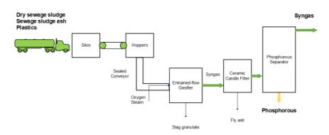
Figure 7. A schematic for the MFC technology-based Niederaussem pilot. Adapted from a presentation by one of the partners in the ITZ-CC project (pilot testing of the MFC technology) [5]
