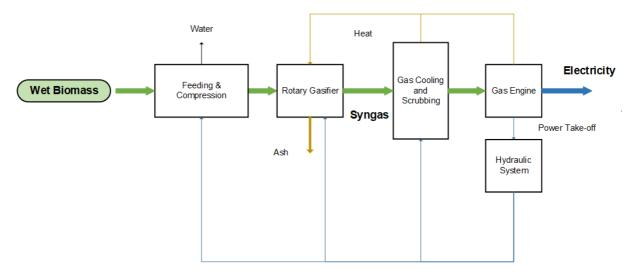
Figure 10. A simplified schematic for SUNY Cobleskill's Inclined Indirect Flaming Pyrolysis Rotary Gasifier based on [1, 2]
