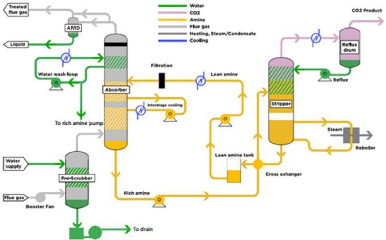
Figure 3. Process diagram of the FOV carbon capture pilot (FOV 2020 webinar). Note: The carbon capture Pilot plant is owned by FOV and was delivered by Kanfa.
