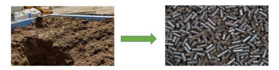
Figure 4. From paper sludge to hydrochar
