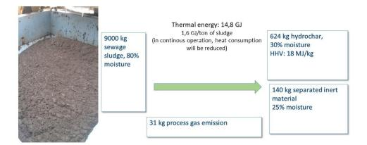
Figure 3. From Sewage sludge to biocharmaterials
