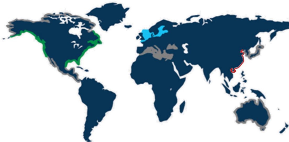
Figure 2.5. IMO world map for emission control areas in 2020. Globally there is a 0.5% sulphur limit. Sulphur emission control areas (SECAs) include the Baltic- and The North sea area (blue) with a 0.1% sulphur limit, the North American ECA (green) with a 0.1% sulphur limit, Chinese National waters (red) additional restrictions for open loop scrubbers, and discussed future ECA (grey) 21 .
