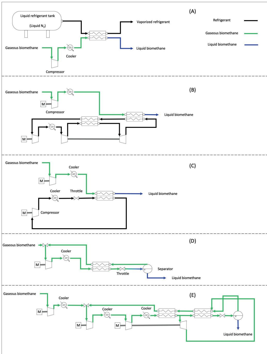
**Figure 8. Biomethane liquefaction:** (A) Liquid nitrogen vaporization, (B) Reverse Brayton cycle, (C) Reverse Rankine cycle, (D) Linde Cycle, and (E) Claude cycle.
