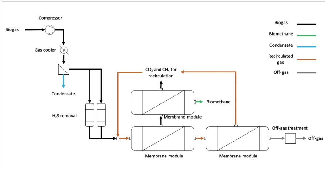
**Figure 6. Membrane separation system topology.**
