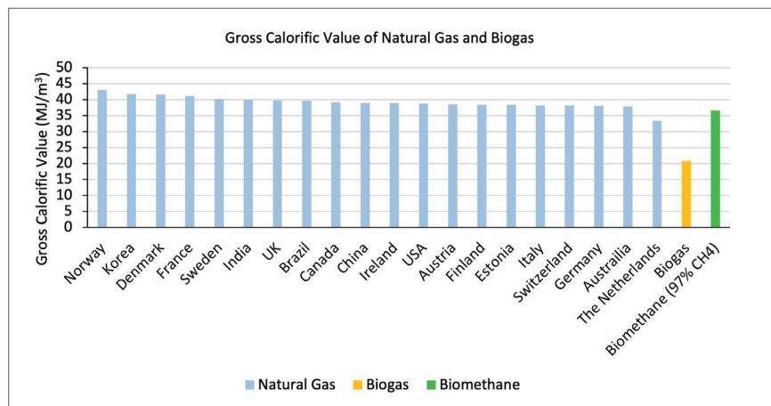
Figure 2. Gross calorific value of natural gas and biogas (55%<sub>vol</sub> CH<sub>4</sub>). Temperature: 15 °C. Pressure: 1.01325 bar. Data adapted from (IEA, 2021).
