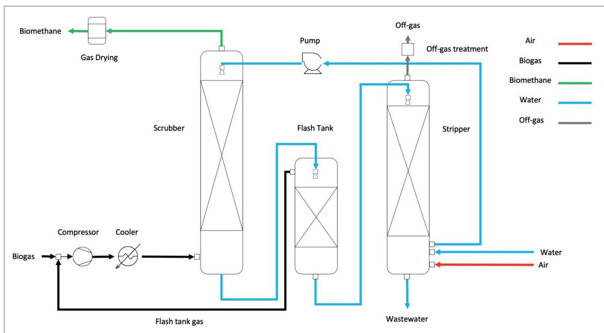
Figure 3. Water scrubbing system topology.
