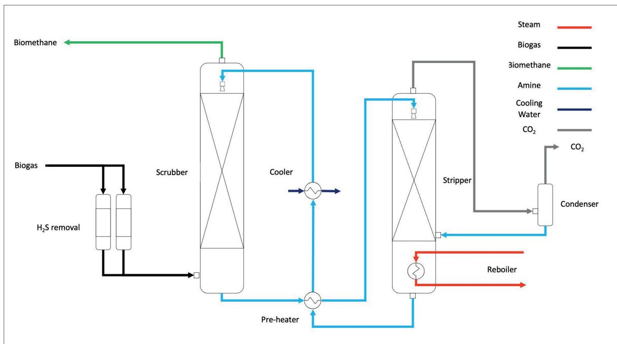
There are combined chemical absorption scrubbers on the market that remove both  $H_2S$  and  $CO_2$  from biogas, that are designed a bit differently to reduce OPEX (mainly developed for the Danish market, where the raw biogas may contain 2000-3000 ppm  $H_2S$ ).
