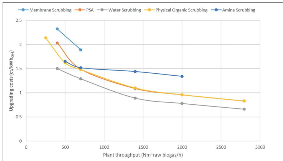
**Figure 19. Specific costs (euro cents) for biogas upgrading technologies.**
