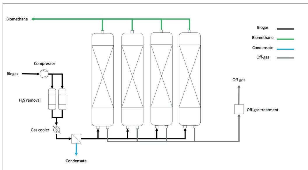
Figure 5. Pressure swing adsorption system topology.
