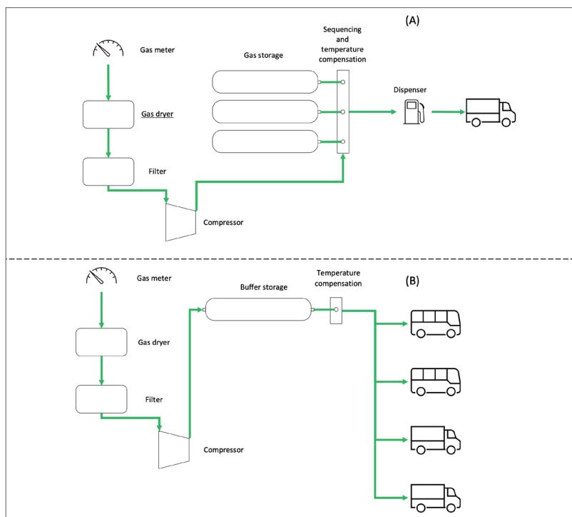
**Figure 11.** (A) Fast fill system (B) Slow fill system.
