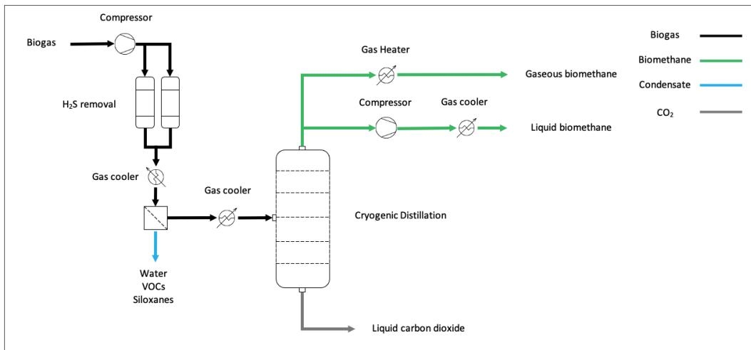
**Figure 7. Cryogenic separation system topology.**
