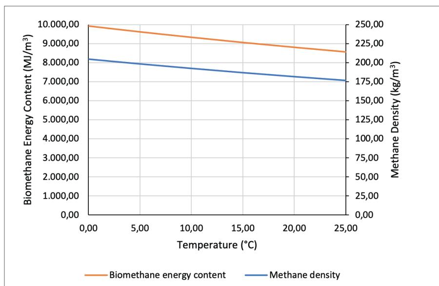
**Figure 12. Impact of temperature on compressed biomethane density and energy content.**
