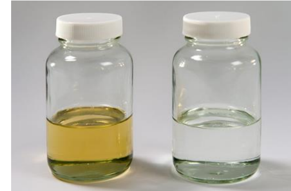
Conventional diesel fuel (left) and F-T ultra pure diesel (right)
