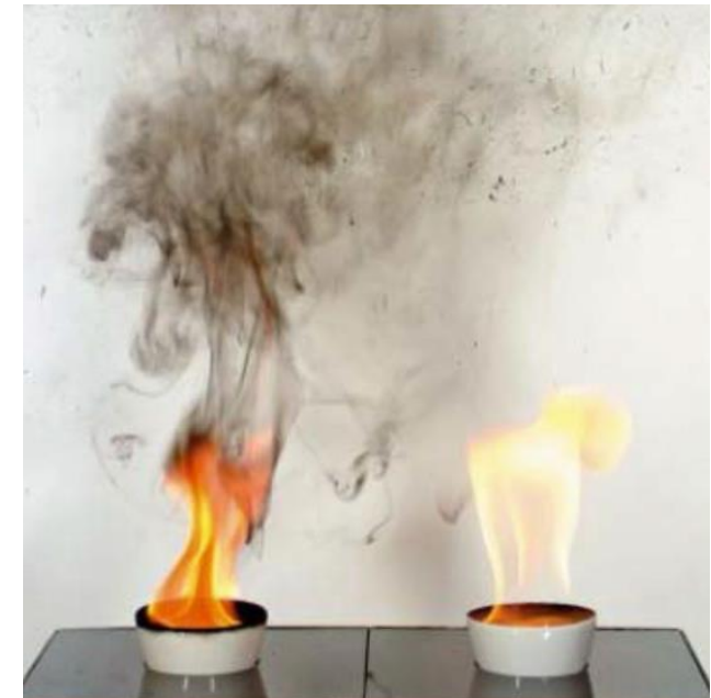
Conventional diesel fuel (left) and F-T ultra pure diesel (right)
