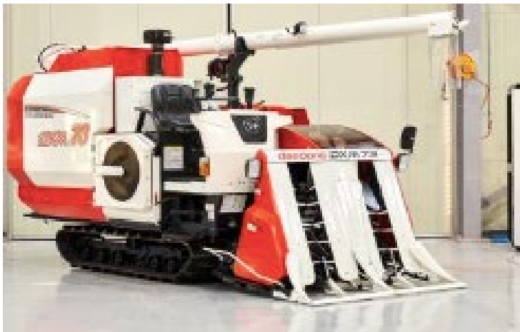
Figure 13: rice and straw co-harvester developed by Straw Innovations. Source: Straw Innovations Ltd
