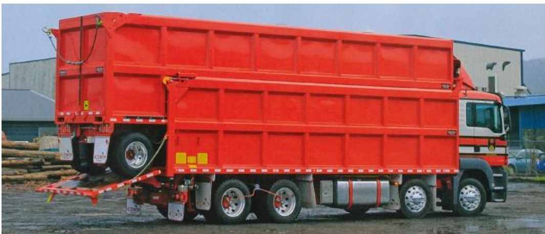
Figure 30b - bin truck and trailer being loaded with bin wood and the same bin truck and trailer unit shown piggy backing its trailer when empty.
