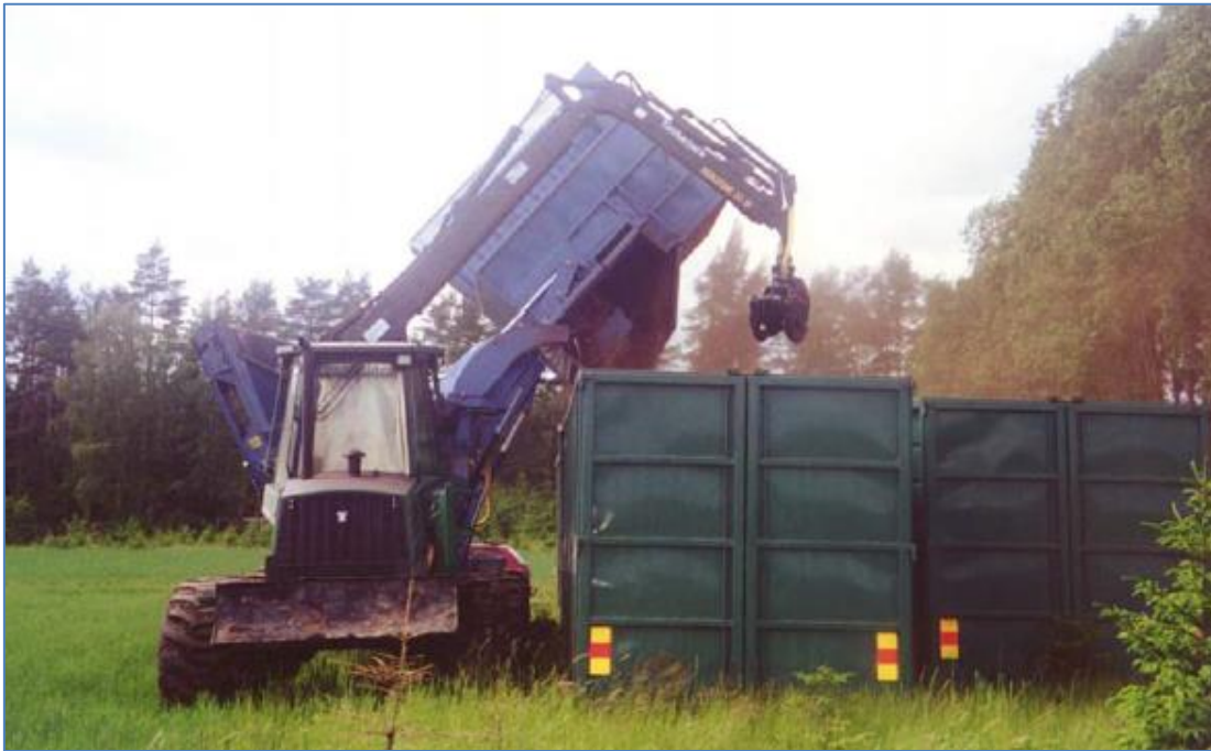
Figure 12 - Chipper forwarder loading set-out bins with chip.
