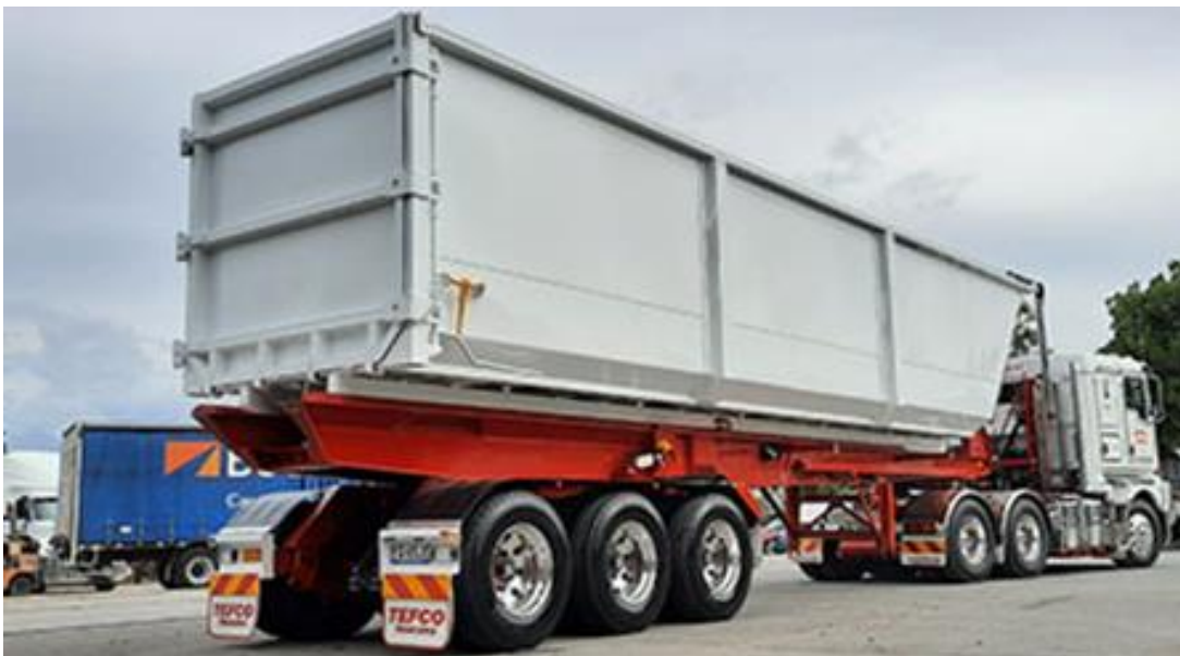
Figure 17 - Set-out bins - hook semi-trailers
