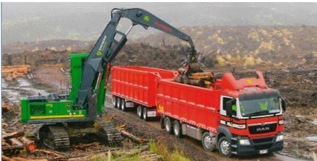
Figure 30a - empty logging truck piggy-backing its trailer
