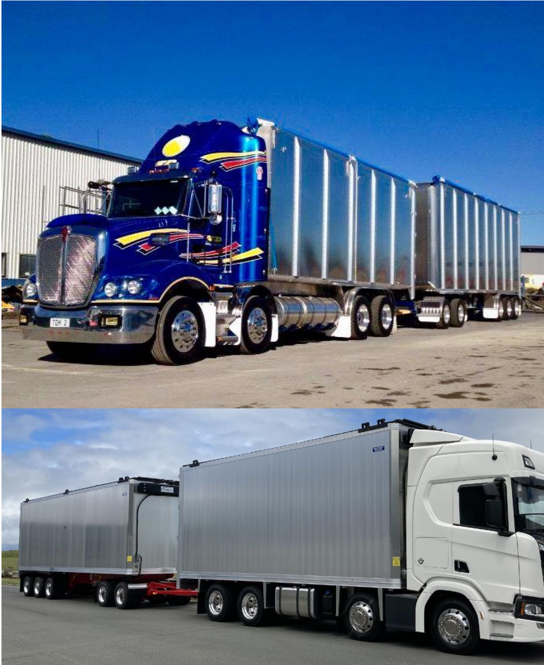
Figure 15 - High volume chip trucks and trailers typically used in New Zealand
