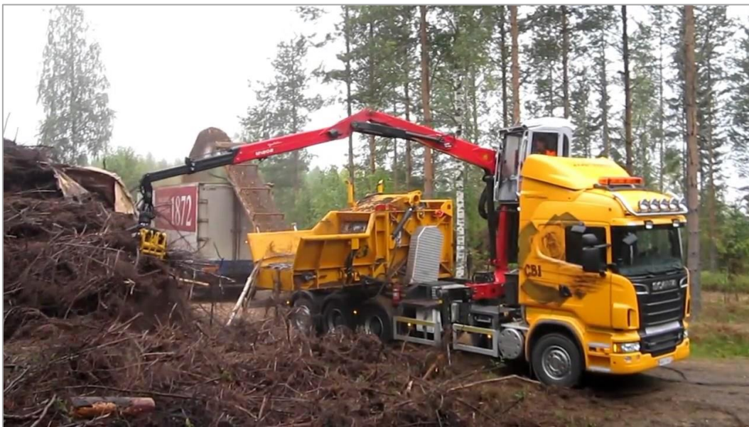
Figure 25 - Truck mounted drum chipper / loader - discharge to truck
