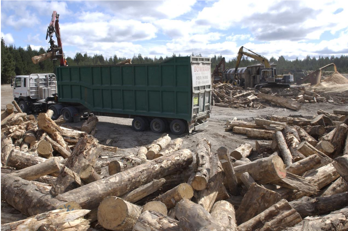
Figure 16 - Bin truck - semi trailer plus self-loader crane
