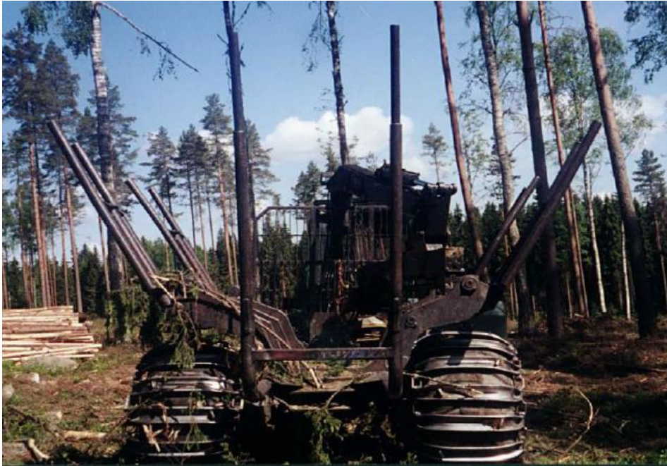
Figure 10 - Forwarder with bunk extended to allow greater load volume
