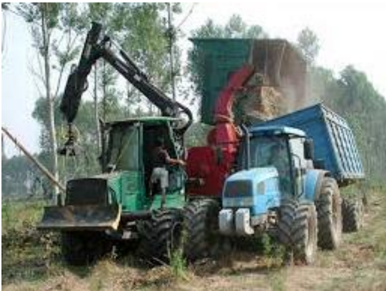
Figure 29 - Chipper forwarder with chip shuttle (Ag-tractor and tipping trailer)
