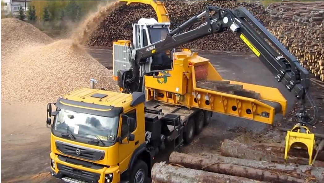
Figure 24 - Truck mounted drum chipper / loader - discharge to ground
