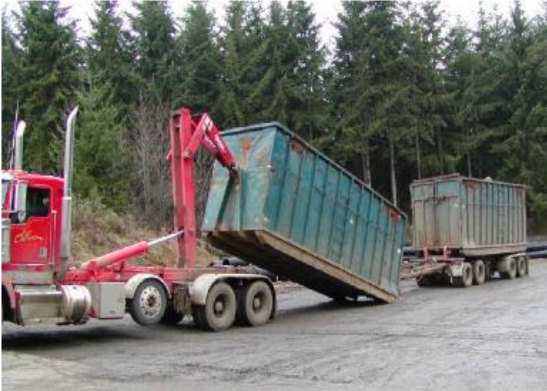
Figure 14 - Truck and trailer unit collecting chip bins
