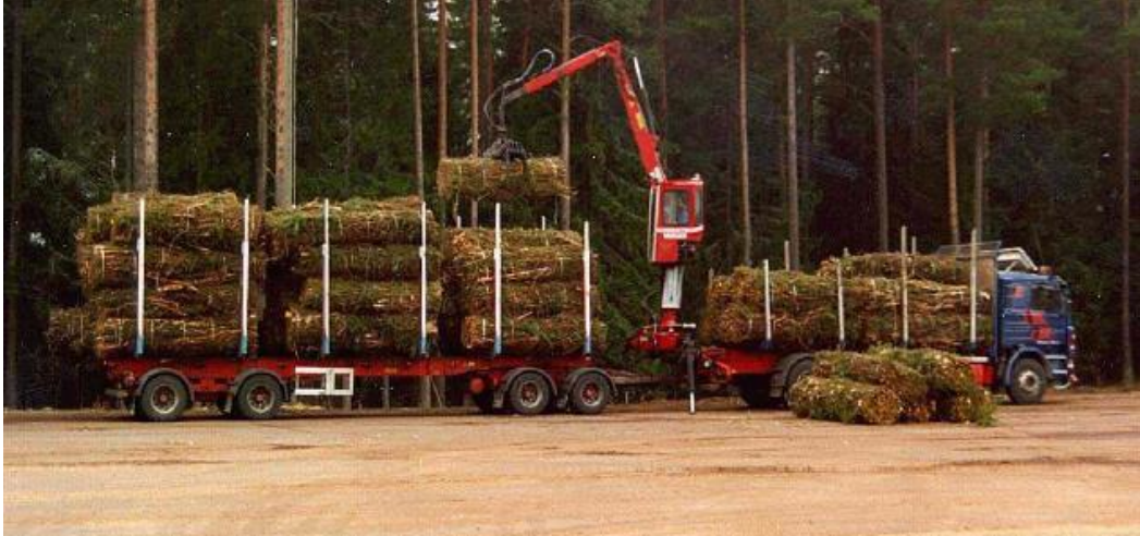
Figure 8 - Conventional log truck and trailers can carry residue bales.
