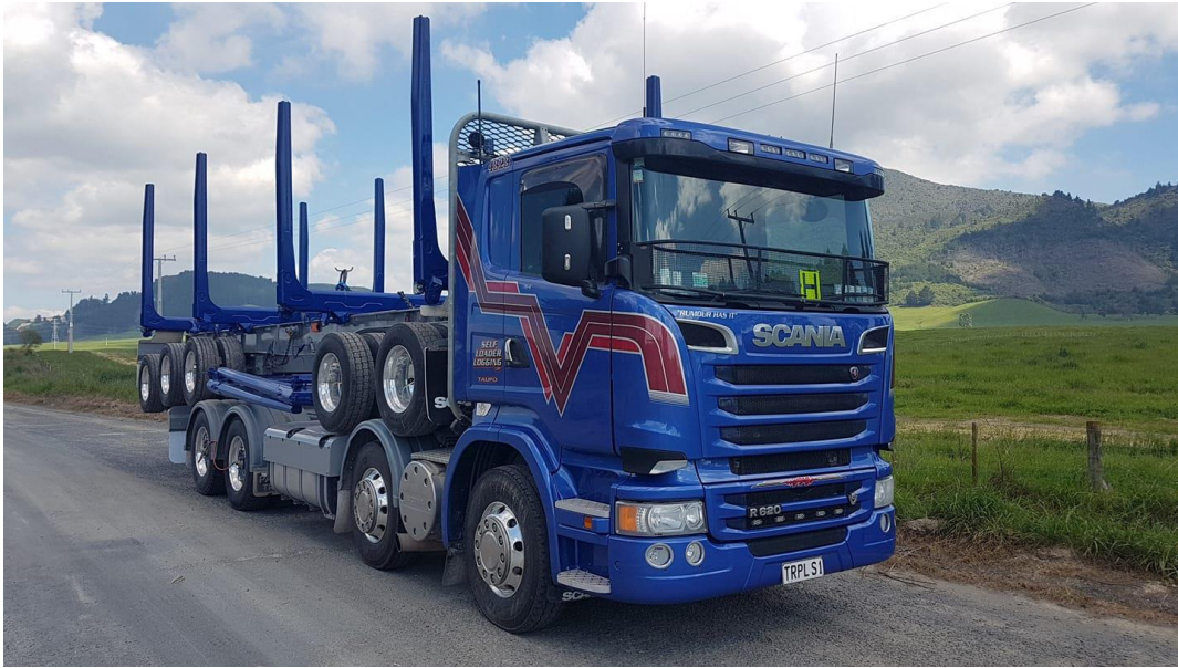
Figure 30a - empty logging truck piggy-backing its trailer
