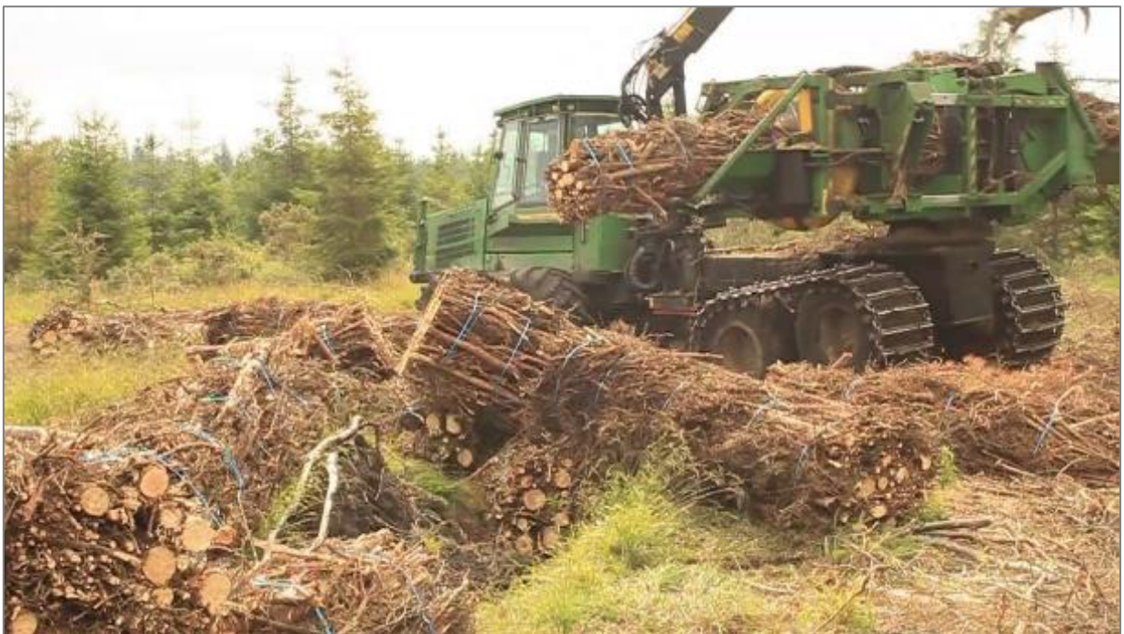
Figure 7 - Residue baler and bales ready for forwarding to roadside.
