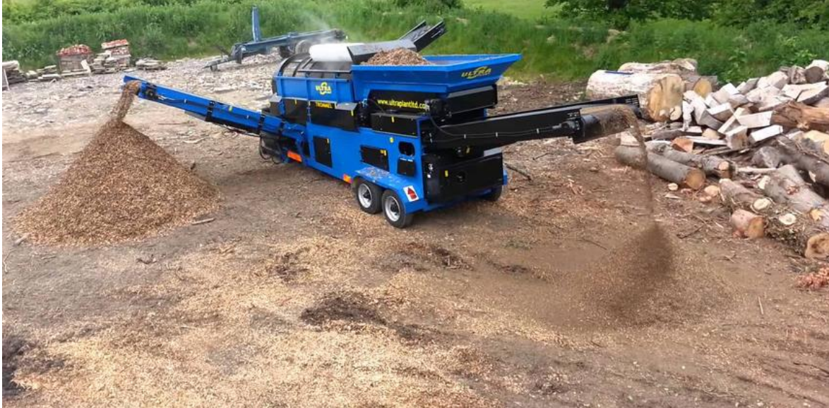
Figure 21 - Mobile trommel screen removing fines from hog fuel
