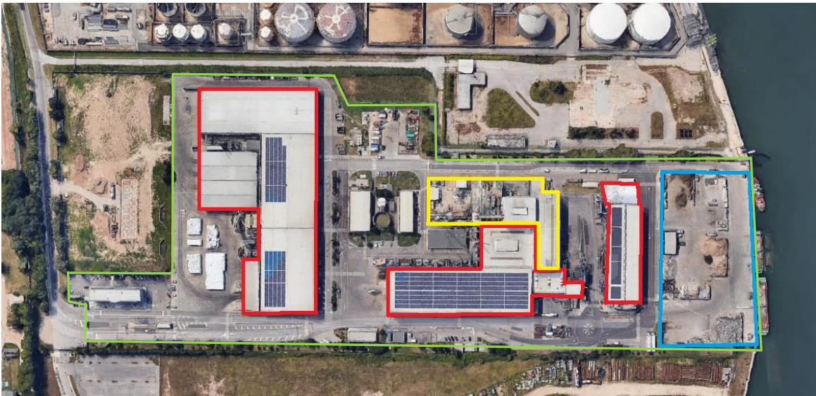
Figure 2. The industrial area of Eco+Eco Srl (in green). The three operational MSW processing areas: transfer area (in blue), SRF production and treatment (in red) and the co-incinerator area (in yellow).
