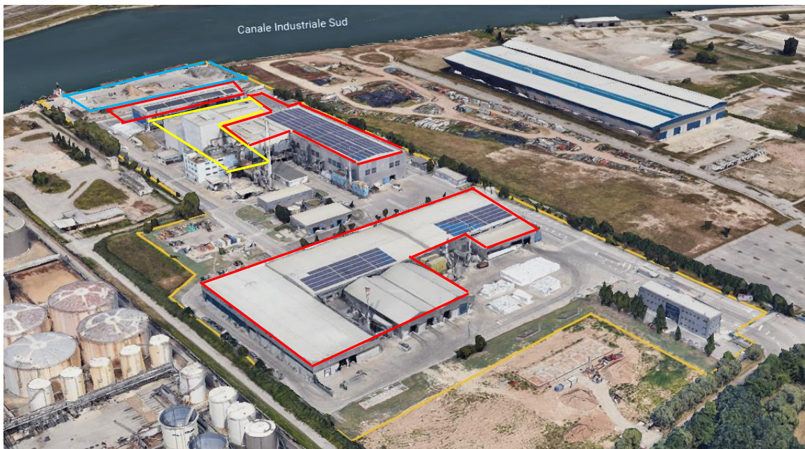
Figure 1. The industrial area of Eco+Eco Srl (in orange). The three operational MSW processing areas are: the transfer area (in blue), the SRF production and treatment area (in red) and the co-incinerator area (in yellow).
