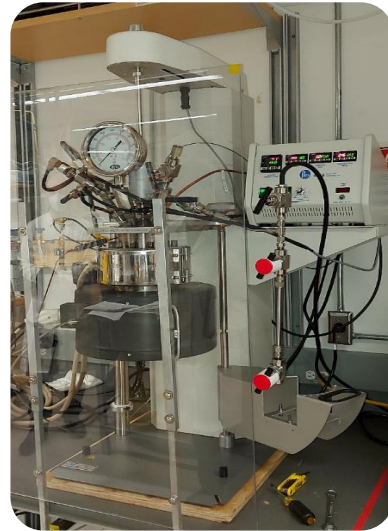
Parr reactor (1-L, CSTR, maximum 500°C, 345 bar)
