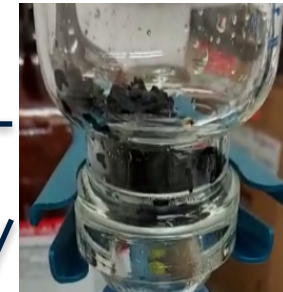
Hydrochar+biocrude retained on filter
