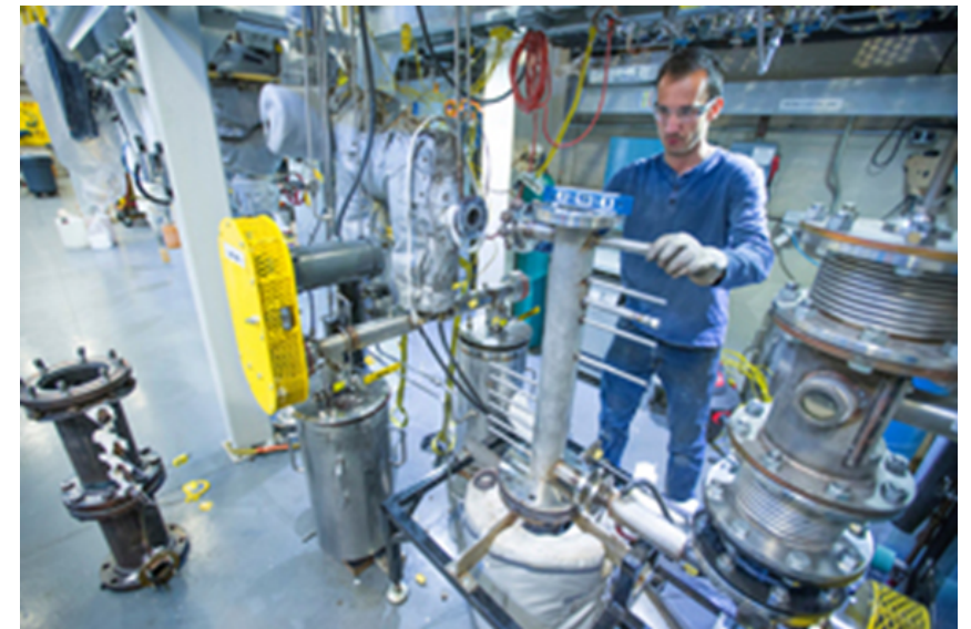
Downsizing pyrolysis vessel (3.5 in vs 6 in dia.) to accommodate higher throughputs achieved with autothermal pyrolysis
